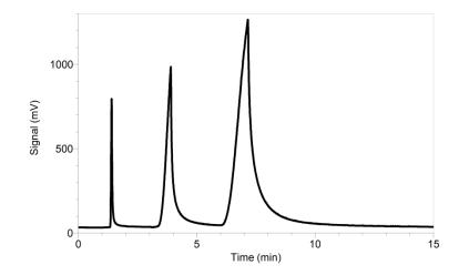
Figure 1. An example of a gas chromatogram showing good separation of three analytes.
