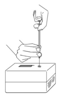
Figure 2. Proper method for injecting a sample into a Vernier Mini-GC.<sup>1</sup>
